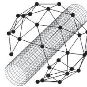
Fig. 4 An illustration of the measuring grid used in our proposal. Each of the points on the imaginary sphere surrounding the cylindrical microphone array represents a direction at which beamforming is carried out to build a spherical pressure distribution. Some points are omitted for clarity, but the measuring grid covers a full sphere around the cylinder.
