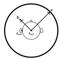
Figure 2. Geometry for near-field HRTF synthesis.
