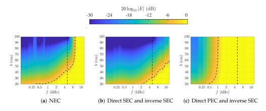
**Figure 7.** Comparison of performance with synthesis error (20) in dB (P = 252, q = 5,  $N_g = 14$ ). (a) synthesis with NEC. Panel; (b) synthesis with direct and inverse SEC; (c) synthesis with direct PEC and inverse SEC.
