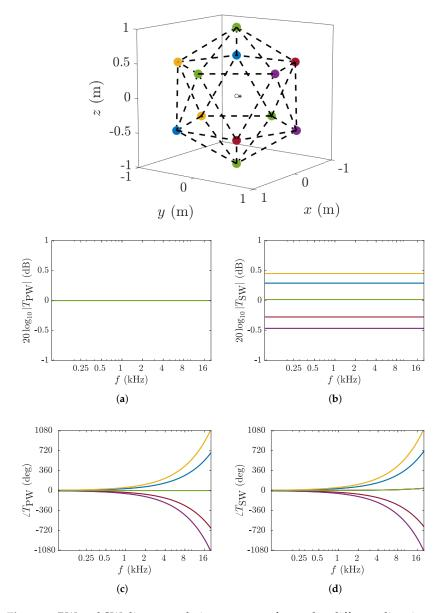
**Figure 6.** PW and SW direct translation operators for twelve different directions along the vertices of the icosahedron (top panel), at a distance of 100 cm from the center of the head. (a) Magnitude in (22); (b) Magnitude in (24); (c) Phase in (23); (d) Phase in (25).
