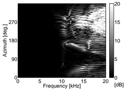
Fig. 9. Spectral distortion of 36 microphones and 8 deg intervals of *controlled directions* (45 directions).
