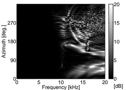
Fig. 12. Spectral distortion of 36 microphones and 4 deg intervals of *controlled directions* (90 directions).
