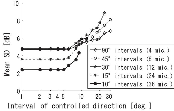
Fig. 8. Relation between the average of spectral distortion and the number of *controlled directions* for each microphone arrangement.
