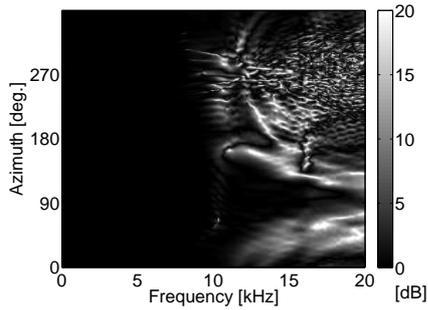
Fig. 11. Spectral distortion of 36 microphones and 5 deg intervals of *controlled directions* (72 directions).
