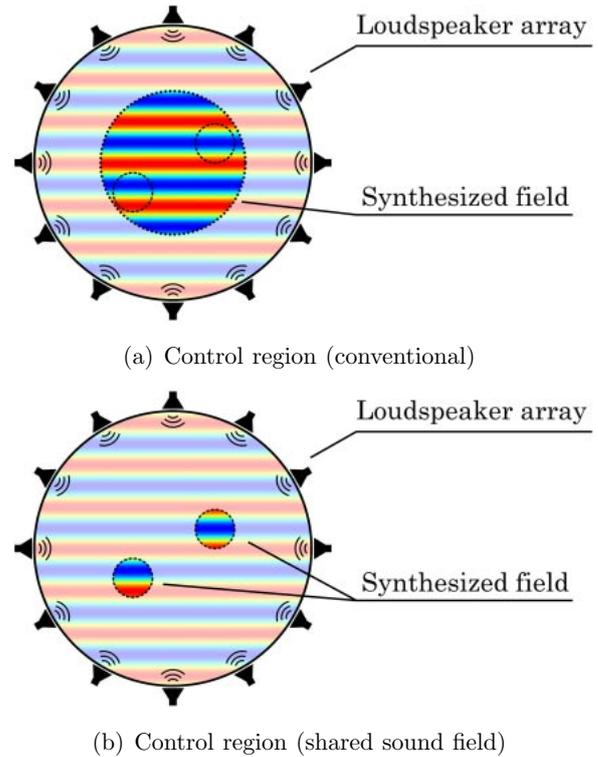
**Fig. 1** (a) Regions to cover multiple listeners, which are controlled during conventional sound field synthesis and (b) the shared sound field synthesis approach. Faint colors show the underlying (target) sound field while bright colors show the reproduction areas.
