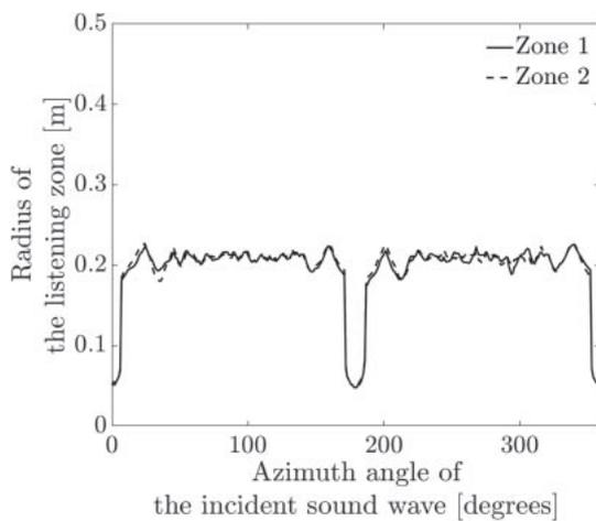
**Fig. 7** Radii of the listening zones as a function of the azimuth angle of incidence. The target source is a 1 kHz plane wave with an incidence direction from an elevation of  $0^\circ$  and the azimuth angle is varied from  $0$  to  $359^\circ$  at intervals of  $1^\circ$ . The two listening positions are located  $-0.5$  and  $0.5$  m away from the center of the loudspeaker array on the  $x$ -axis, respectively. The number of time instants is 5.
