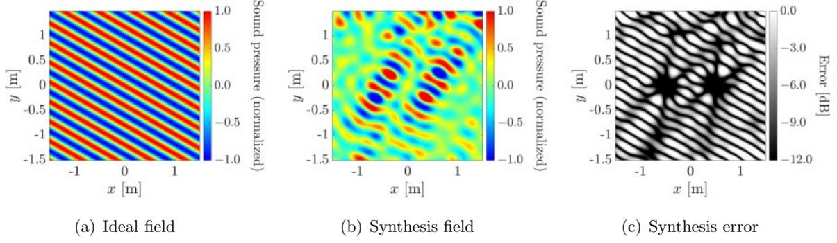
**Fig. 5** Sound pressure field obtained using the proposed method with two-zone synthesis of a 1 kHz plane wave with incidence direction from  $60^\circ$  azimuth and  $0^\circ$  elevation at  $\alpha = 0$ . The two listening positions are located  $-0.5$  and  $0.5$  m away from the center of the loudspeaker array on the  $x$ -axis, respectively.
