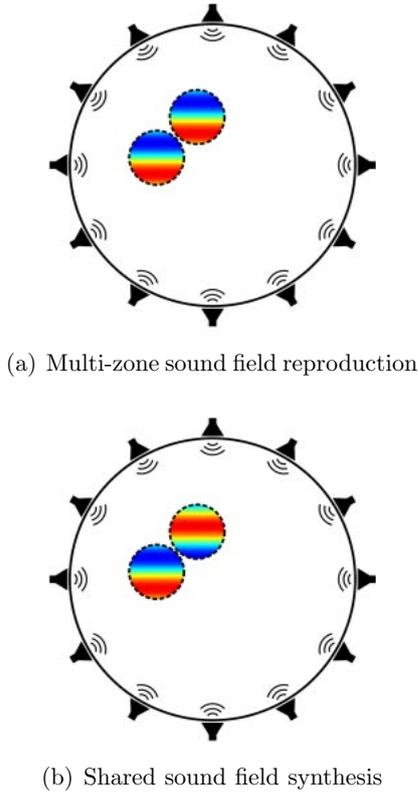
**Fig. 2** (a) The comparison of the synthesis of multiple fields through the conventional multi-zone approach and (b) the shared sound field synthesis approach. The fields obtained by the conventional multi-zone sound field reproduction may lead to unnatural jumps in sound pressure when the fields are close to each other (a), while such a jump is not observed with the assumption of a shared field (b).
